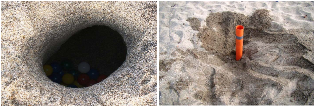
Figure 7. a. False nest elaborated using plastic balls. b. Set up used to measure water table level at both surveyed beaches.
